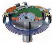
All models are equipped with market-proven absolute encoders. Advanced coding and digital processing technologies provide long-term reliability in any work-site conditions. The 1" and 2" high-precision models incorporate IACS (Independent Angle Calibration System) to further enhance measurement reliability.
